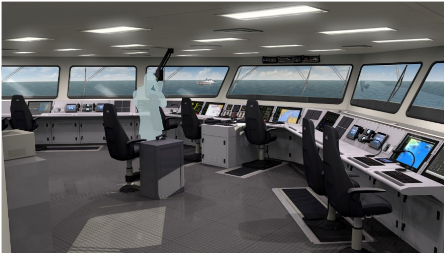
Artist Rendering of OSI Maritime Systems’ Integrated Bridge Management System for the F126 Program
